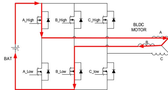
Fig. 3. Motoring Current Flow for a Commutation Sequence (Adapted from [10])
