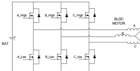
Fig. 2. Power Inverter Circuit (Adapted from [10])
