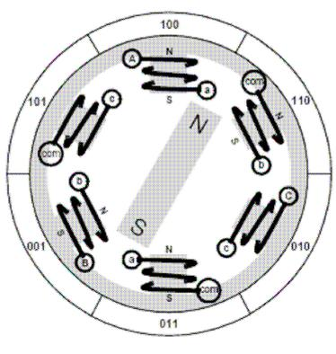
Fig. 1. Permanent Magnet BLDC Construction [4]
