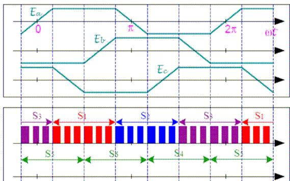
Fig. 4. BLDC EMF with Corresponding Switch Sequence [9]
