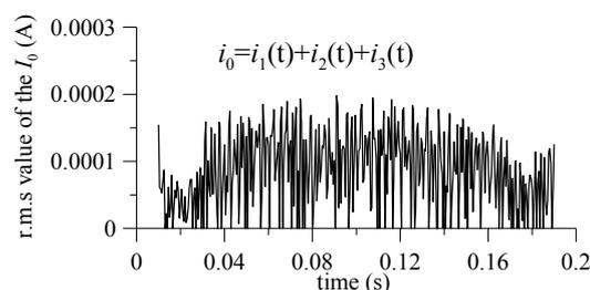
Fig. 5. Controlling the accuracy of currents computation on Fig. 4 - stepping rms value of the stator phase currents sum as a function of time for the locked-rotor operation.
