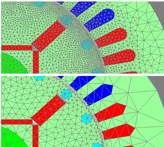
Fig.1 Different options of the mesh discretization in the FEM model.
