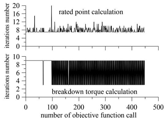
Fig. 6. The Number of iterations associated with obtaining the rated operation point (upper), and the breakdown E-M torque (lower) for subsequent calls of the objective function.
