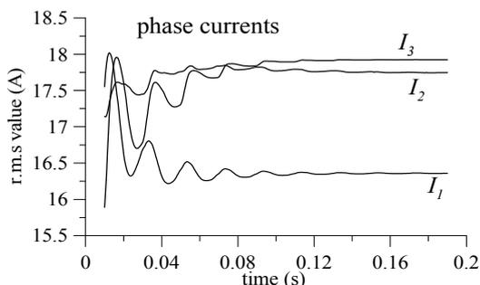
Fig. 4. Stepping rms value of stator phase currents as a function of time for the locked-rotor operation.
