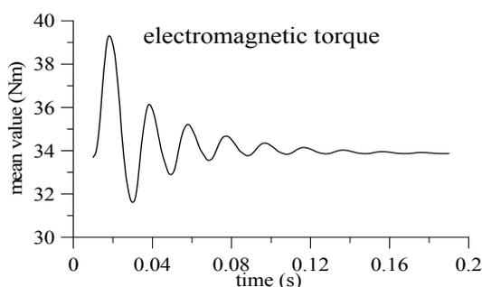
Fig. 3. Stepping mean value of the electromagnetic torque as a function of time for the locked-rotor operation.
