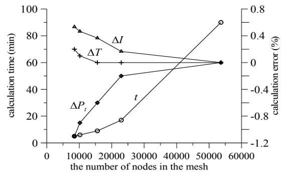
Fig.2 A relationship between computation time  $t$  and percentage errors  $\Delta P_t$  (iron losses),  $\Delta I$  (stator current),  $\Delta T$  (electromagnetic torque), and the number of mesh nodes.
